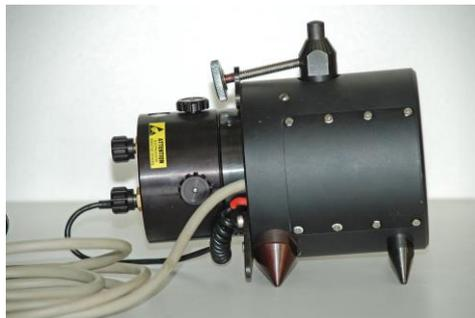
Figure. The adjustable laser source (PS-125)
