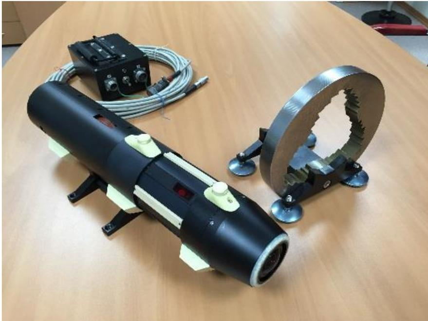
Figure: The PS-120/154 (long version) system without transport box
